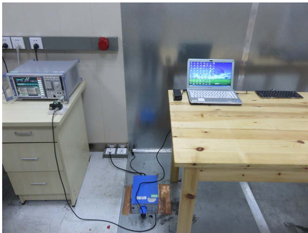
FCC RADIATED EMISSION TEST SETUP
