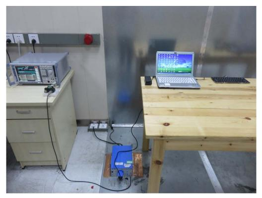
FCC RADIATED EMISSION TEST SETUP
