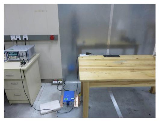
FCC RADIATED EMISSION TEST SETUP
