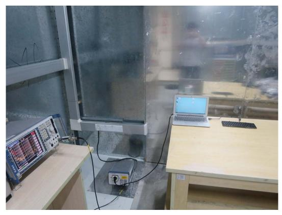
FCC RADIATED EMISSION TEST SETUP
