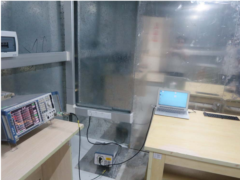
FCC RADIATED EMISSION TEST SETUP
