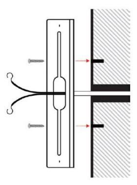
4. Connect the existing doorbell wires to the leads on the back panel of the doorbell.
