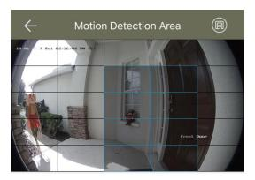
Only receive notifications if an object enters the view of the camera that is highlighted. Adjust the motion detection area by selecting desired grey boxes.
