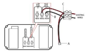
4. Remove the paper backing and adhere the power booster and screw terminal to the mechanical chime. Replace the cover on the mechanical chime.
