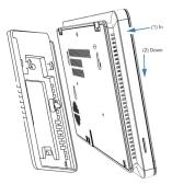
Press the panel onto the mounting bracket, and then slide the panel downward.
