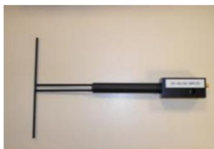
Figure 1 – Satimo COMOSAR Validation Dipole
