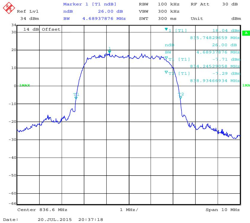
**99% Occupied Bandwidth for HSUPA (BPSK) Mode**
