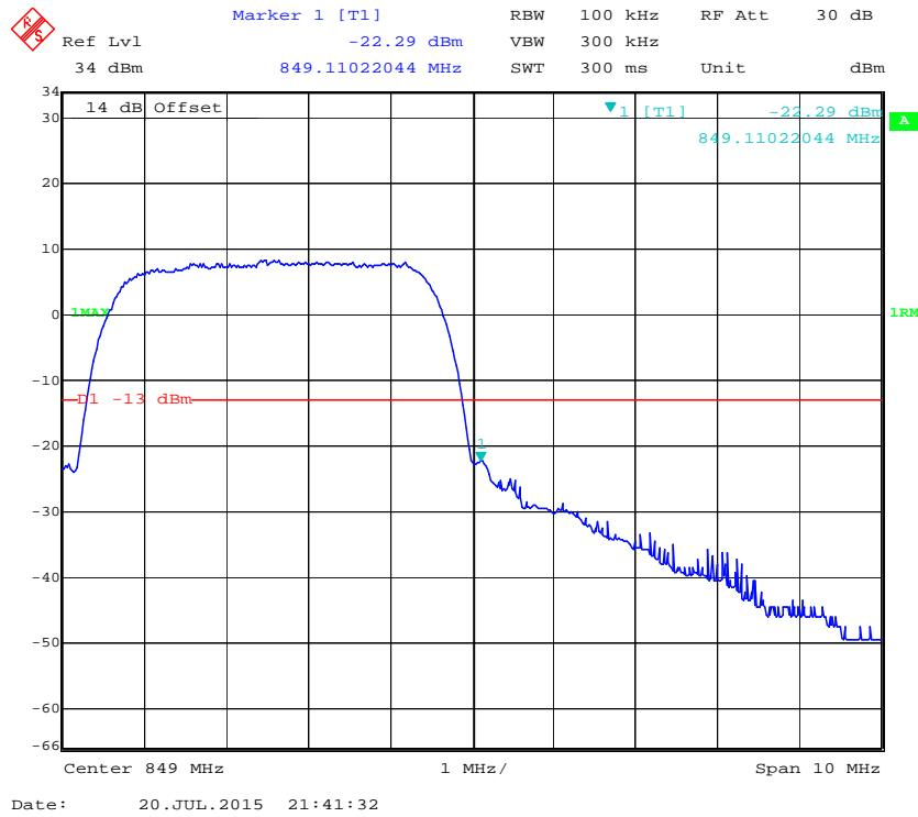
**Cellular Band, Left Band Edge for HSUPA (BPSK) Mode**
