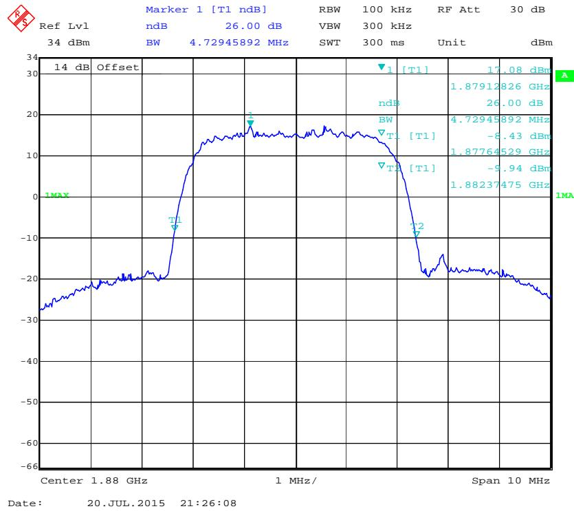
**99% Occupied Bandwidth for HSUPA (BPSK) Mode**
