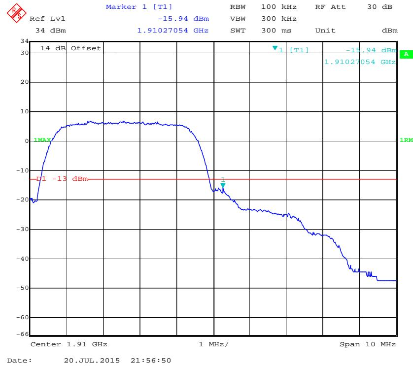
**PCS Band, Left Band Edge for HSUPA (BPSK) Mode**
