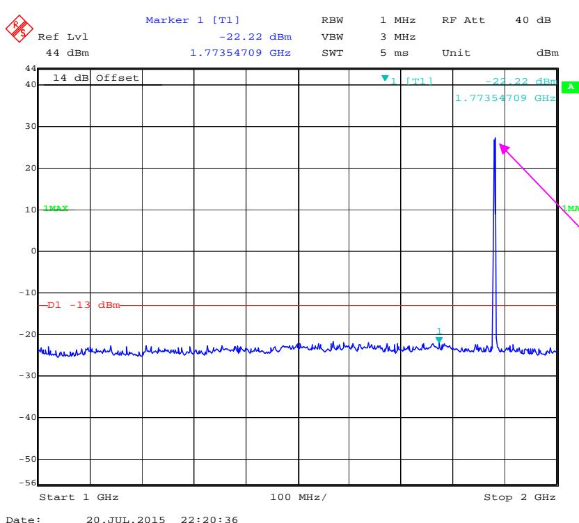
Fundamental test without notch filter
