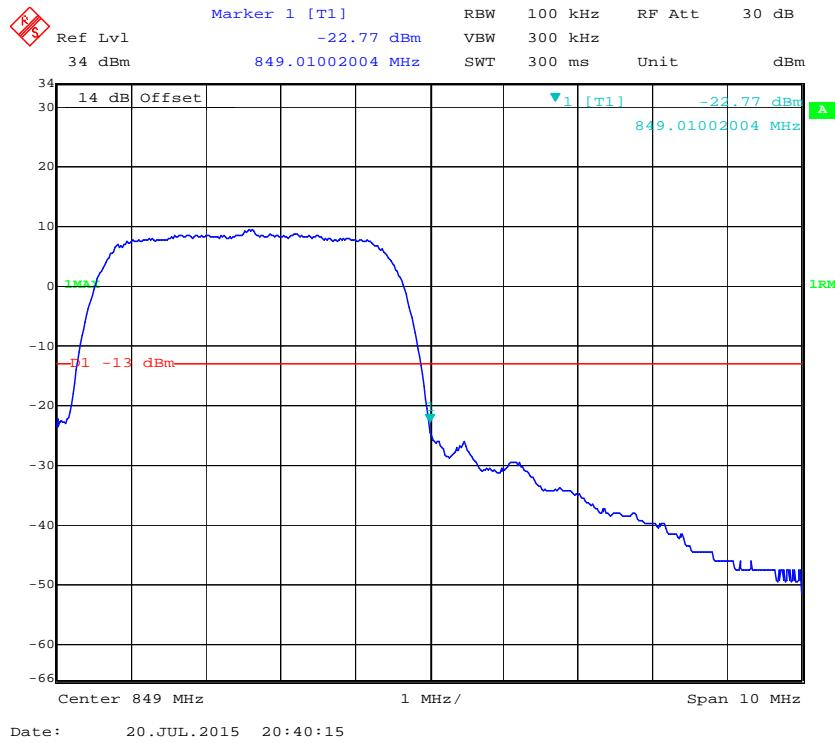
**Cellular Band, Left Band Edge for HSDPA (16QAM) Mode**
