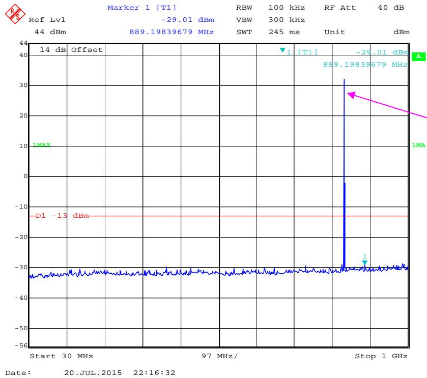
Fundamental test without notch filter
