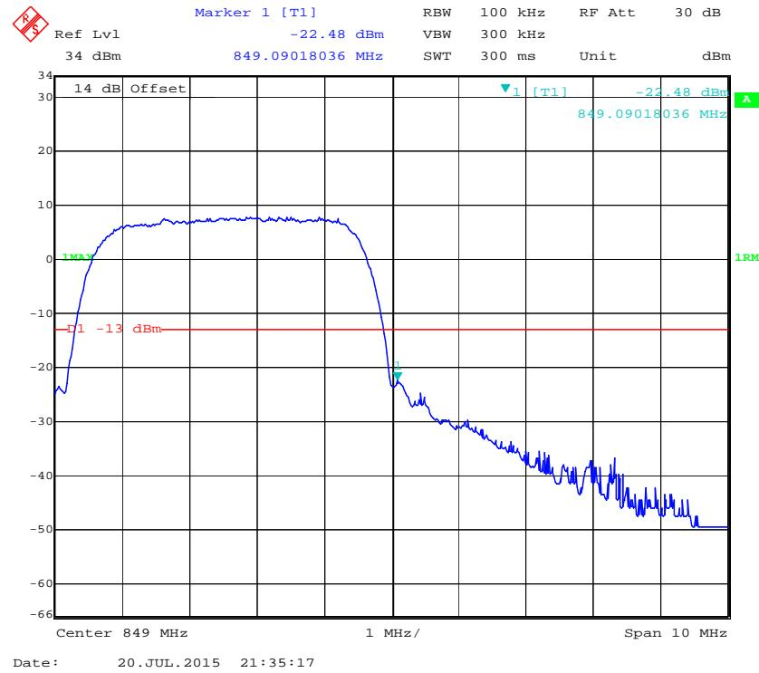
**PCS Band, Left Band Edge for GSM (GMSK) Mode**
