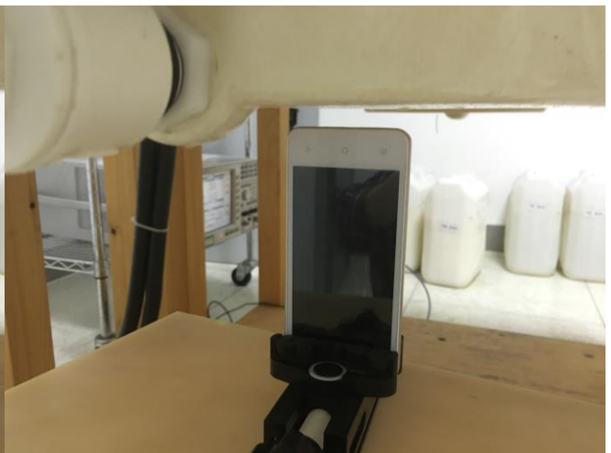
Bottom of the EUT with 1 cm Gap
