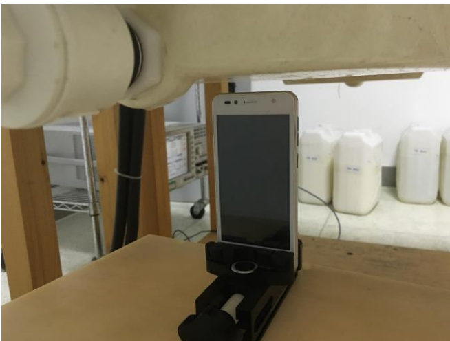
Top of the EUT with 1 cm Gap
