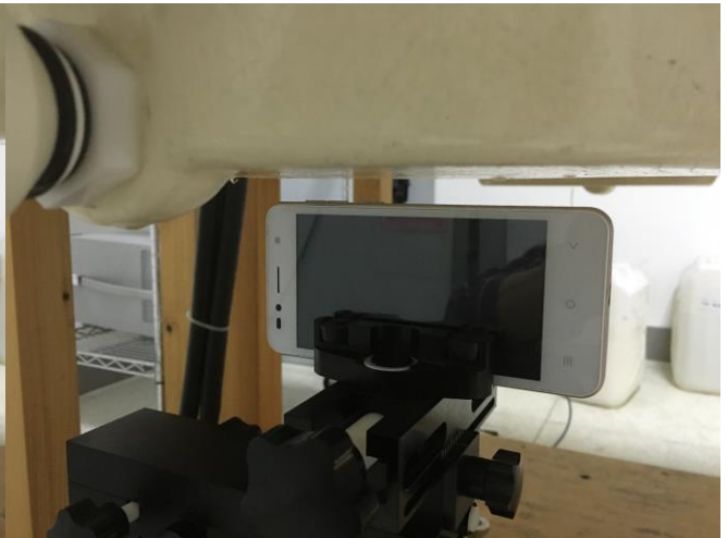
Right Side of the EUT with 1 cm Gap
