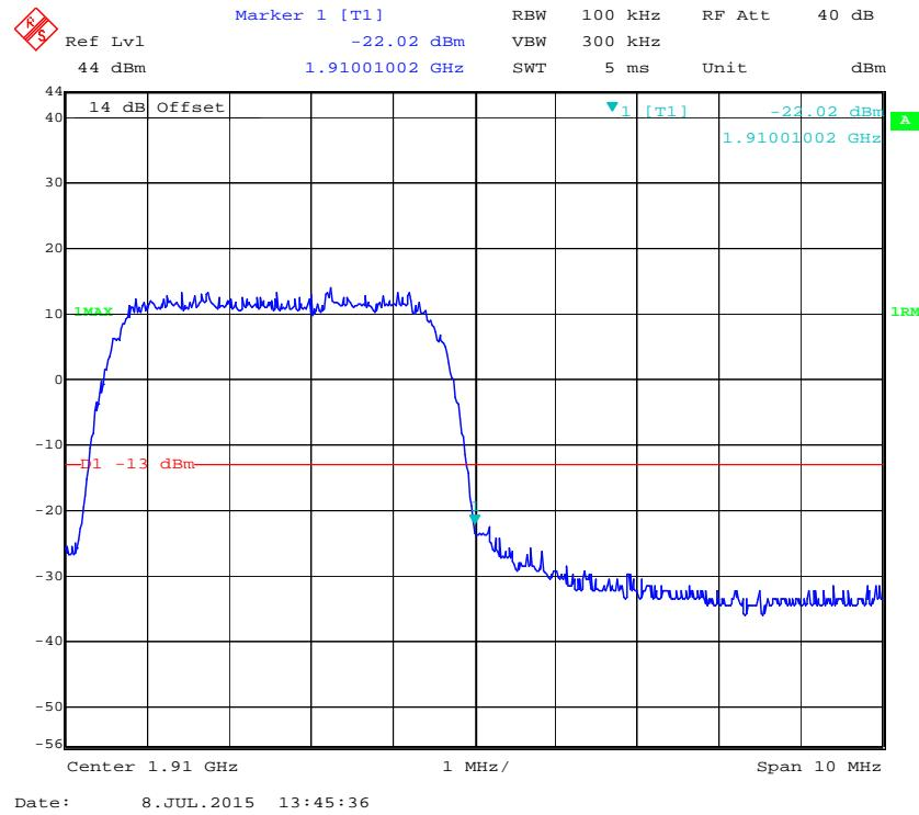
**PCS Band, Left Band Edge for HSDPA (16QAM) Mode**
