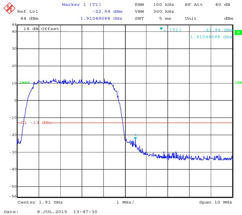
**PCS Band, Left Band Edge for HSUPA (BPSK) Mode**
