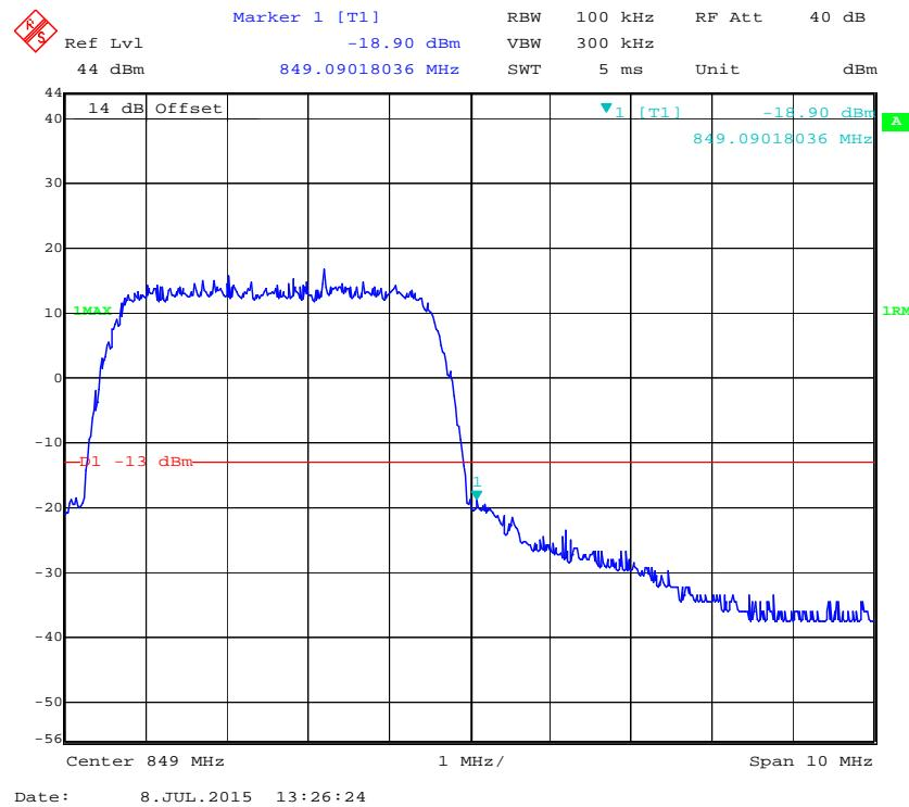
**Cellular Band, Left Band Edge for HSUPA (BPSK) Mode**
