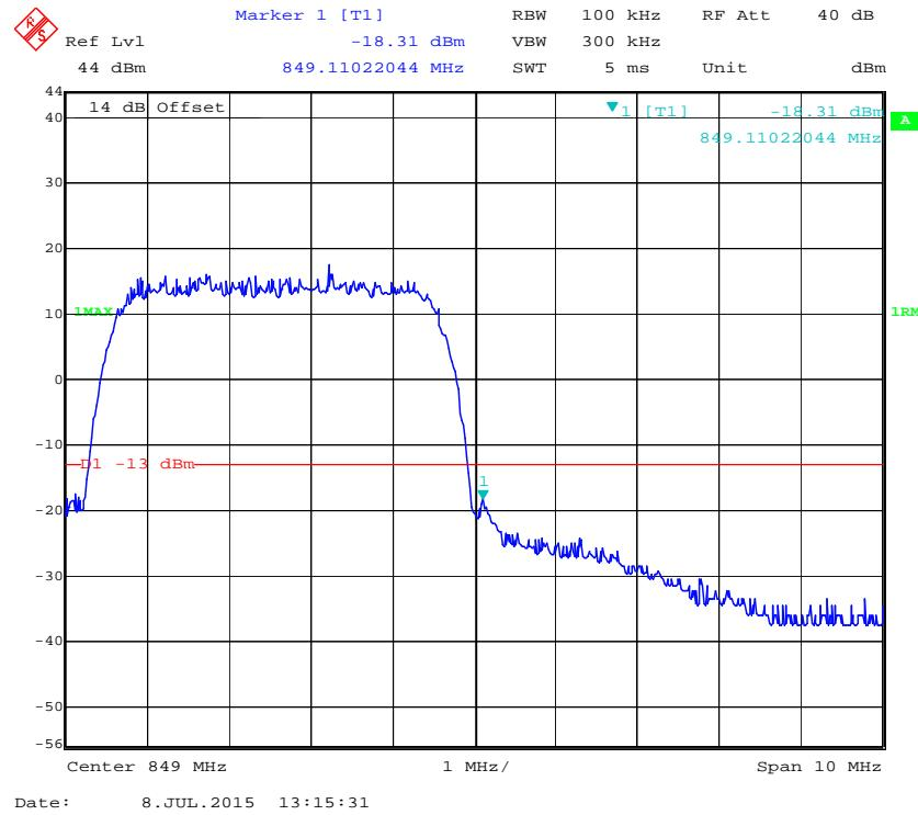
**Cellular Band, Left Band Edge for HSDPA (16QAM) Mode**
