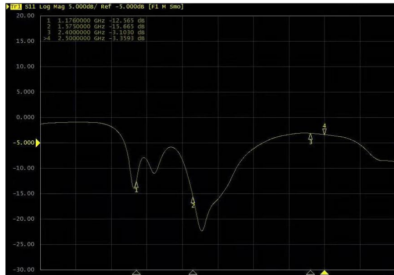
Fig. 2 S11 Parameter-GPS L1/L5 and BT test result
