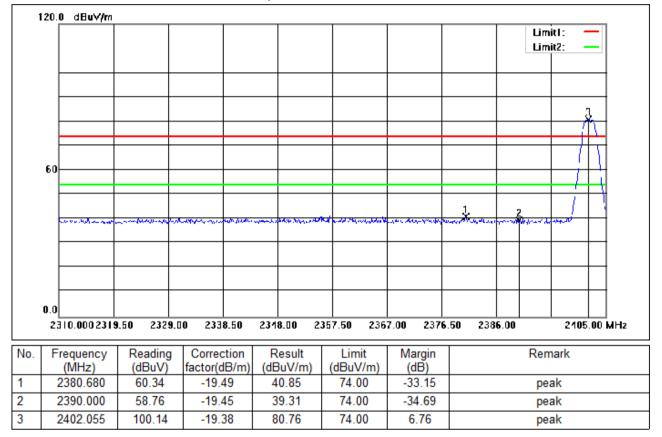
Test Mode: 03; Polarity: Vertical; Modulation:GFSK; Channel:Low
