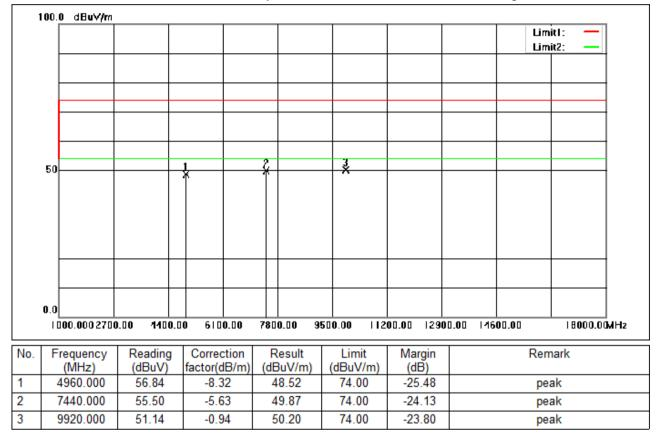
Test Mode: 03; Polarity: Vertical; Modulation:GFSK; Channel:High
