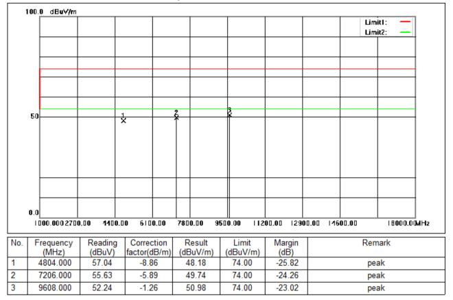
Test Mode: 02; Polarity: Horizontal; Modulation:GFSK; Channel:Low
