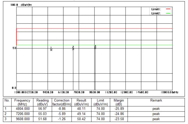
Test Mode: 03; Polarity: Horizontal; Modulation:GFSK; Channel:Low
