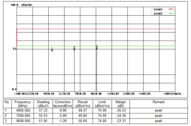
Test Mode: 02; Polarity: Vertical; Modulation:GFSK; Channel:Low
