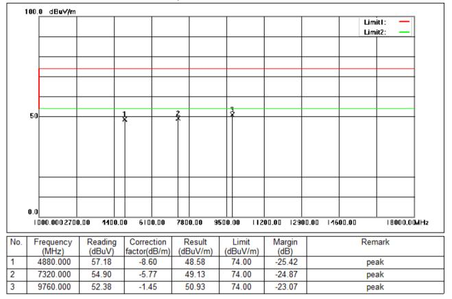
Test Mode: 03; Polarity: Vertical; Modulation:GFSK; Channel:middle
