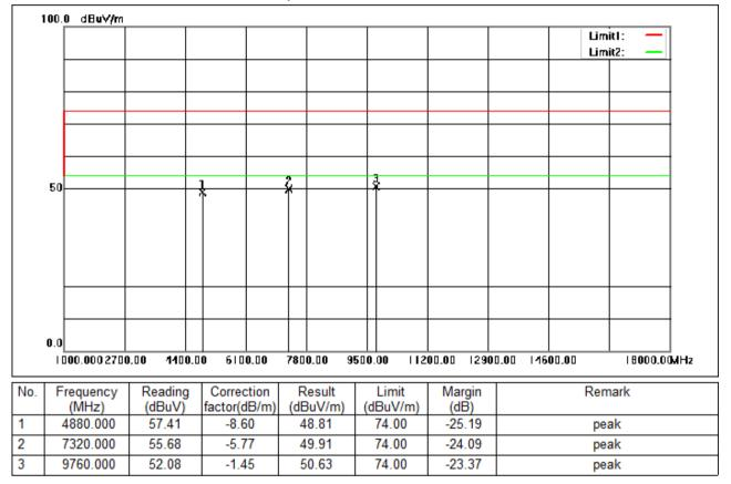
Test Mode: 02; Polarity: Vertical; Modulation:GFSK; Channel:middle
