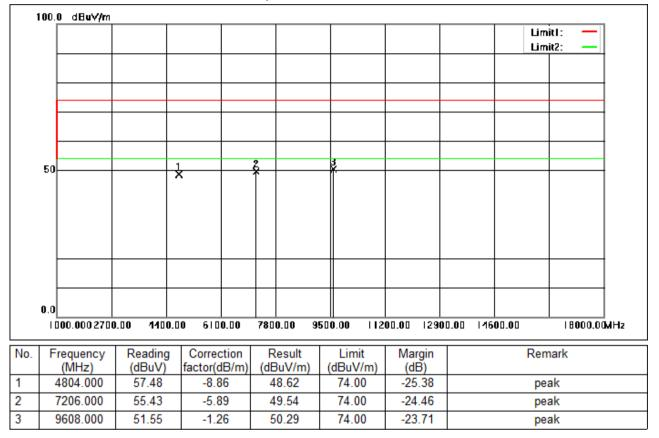
Test Mode: 03; Polarity: Vertical; Modulation:GFSK; Channel:Low
