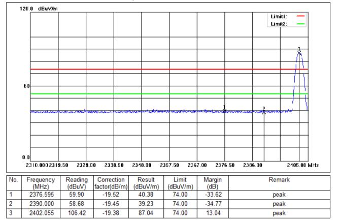
Test Mode: 02; Polarity: Horizontal; Modulation:GFSK; Channel:Low
