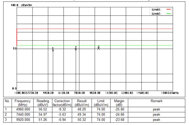
Test Mode: 02; Polarity: Horizontal; Modulation:GFSK; Channel:High
