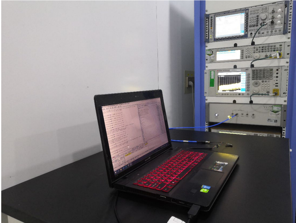
RF Conducted Test setup
