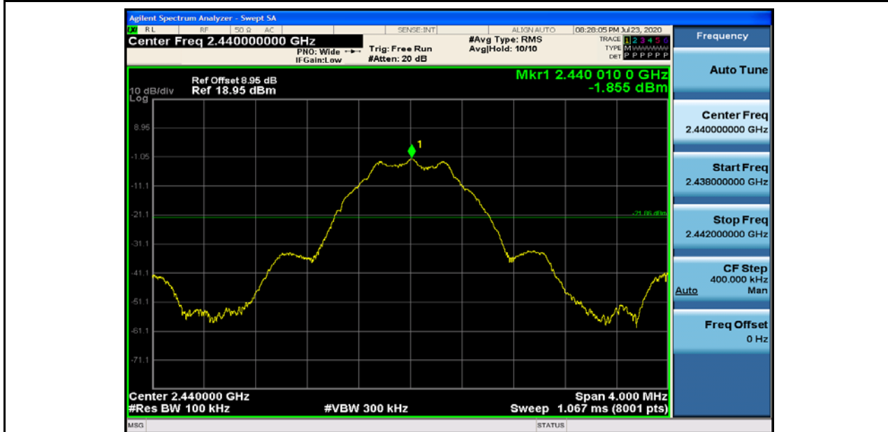
RF Conducted Spurious Emissions_BLE_2440(1M Rate)
