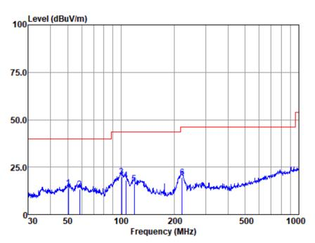
Antenna Polarity : HORIZONTAL EUT/Project :19859CR
