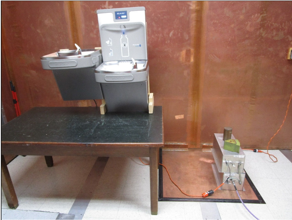
Test Setup for Powerline Conducted Emissions (AC Mains)
