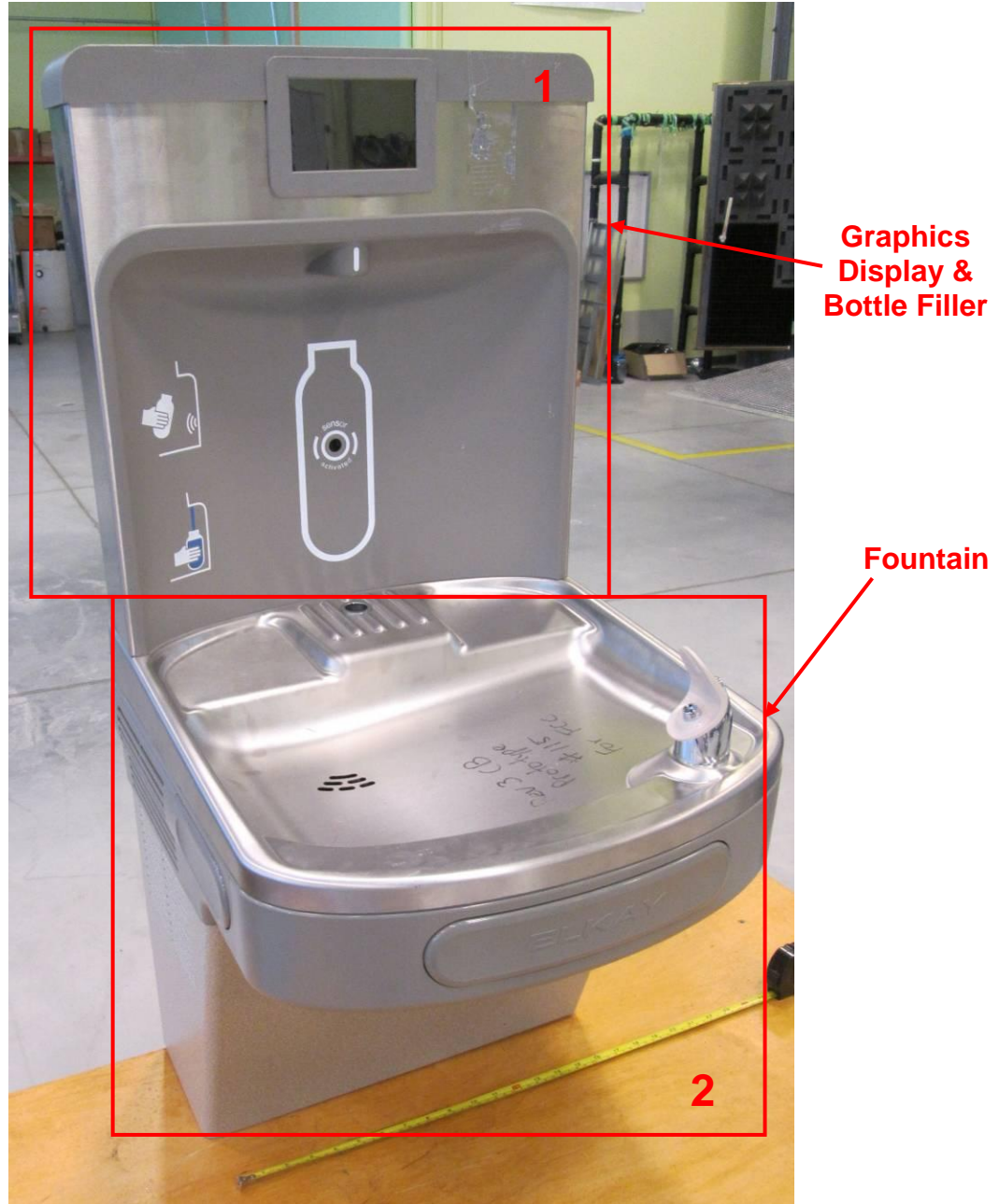
Photo 2. EUT – External view, side 1 Fountain Base 1 containing control board, & connected to Graphics Display
