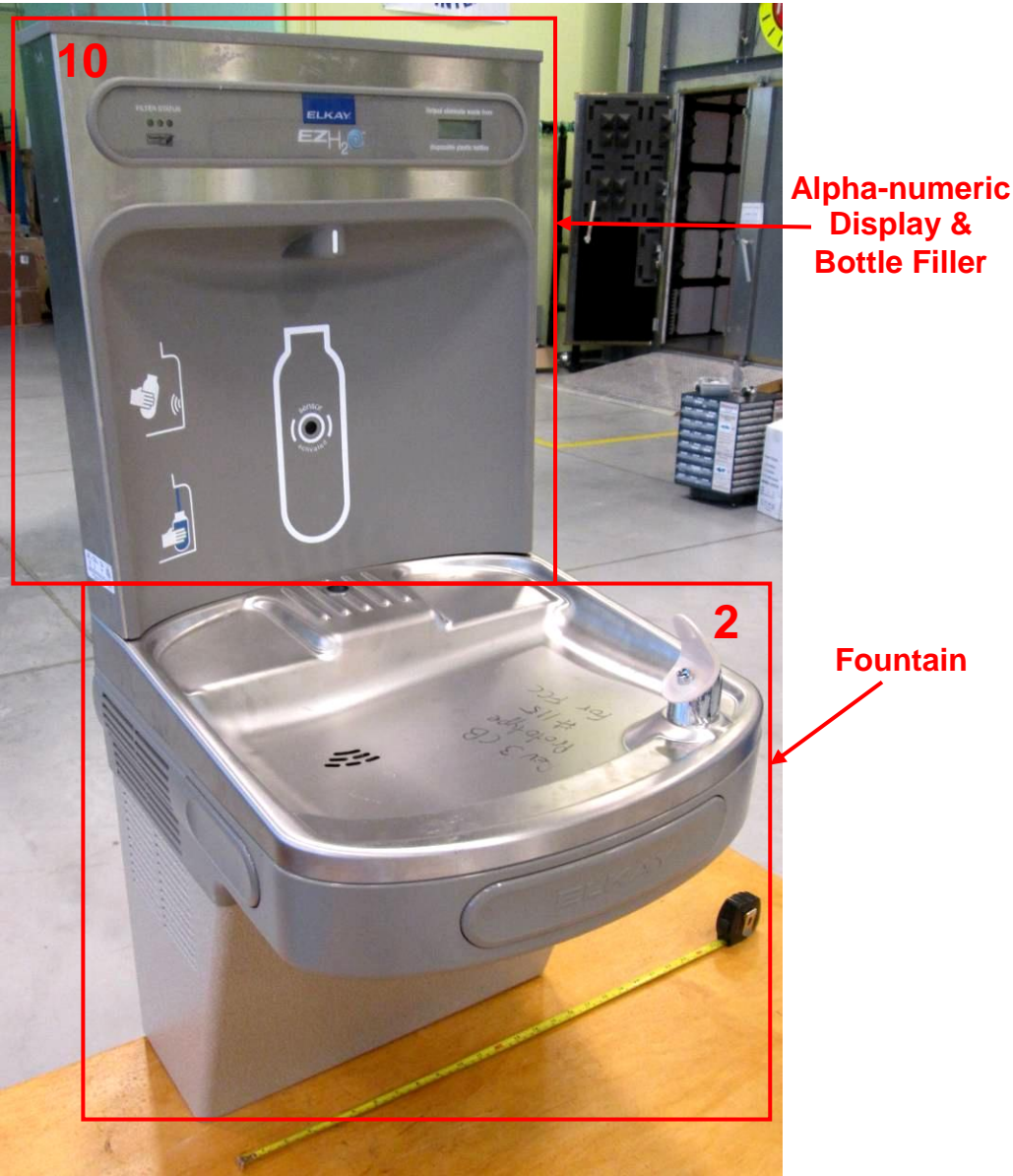
Photo 6. EUT – External view, side 1 Fountain Base 1 containing control board, & connected to Alpha-numeric Display (back view is identical to photo #3)
