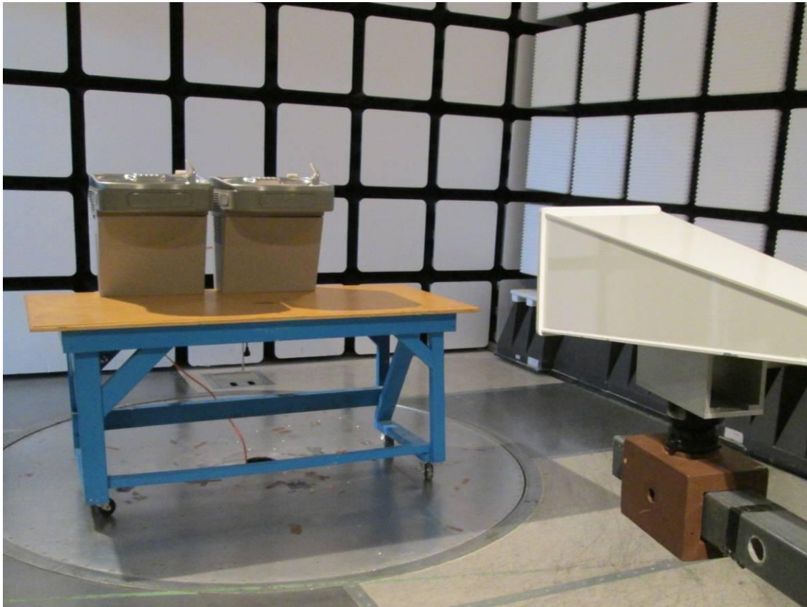
Photo 3. Radiated Emissions 3 Testing on RF boards. Setup for unit with Graphics Display and Alpha-numeric Display are similar.
