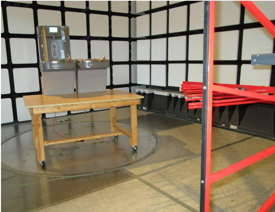
Photo 2. Radiated Emissions 2 Testing on unit with Graphic Display connected. Setup for unit with Alpha-numeric Display and RF testing are similar.
