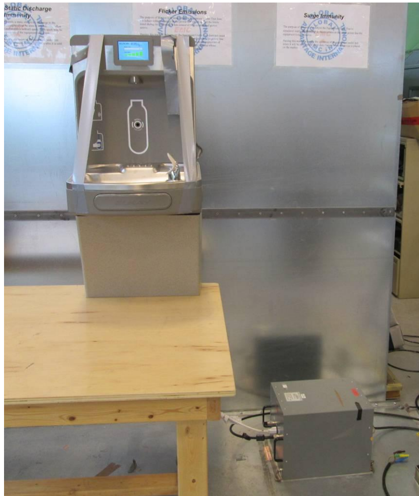
Photo 5. Power Line Conducted Emissions Testing on unit with Graphics Display connected. Setup for unit with Alpha-numeric Display is similar. Both the 900 MHz and 13.56 MHz boards are incorporated into this unit, and test is performed with both RF on for both displays.
