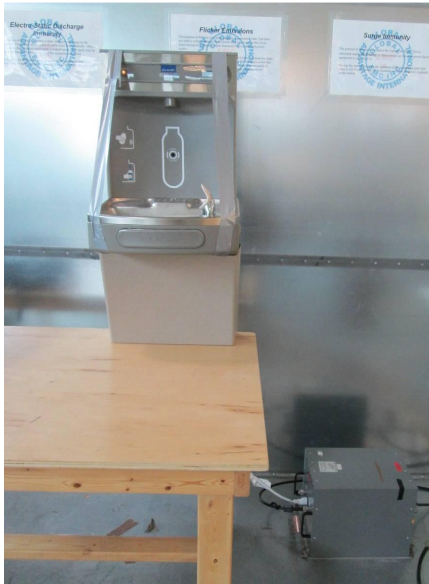
Photo 5. Power Line Conducted Emissions Test is performed with RF on.
