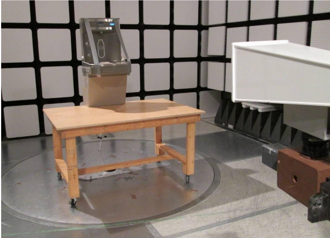
Photo 2. Radiated Emissions 2 Setup with Alpha-numeric Display connected. RF testing is similar.
