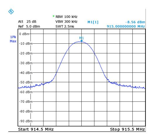
Mid Channel Note: 20 dB for external attenuation losses added to value shown above.
