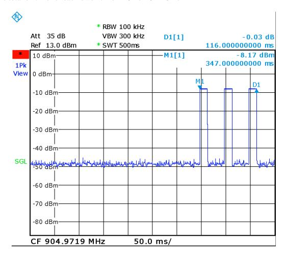
(On time for each transmission) x (Maximum number of transmissions in 20s)  $= 45 \text{ms} \times 3 = 135 \text{ms} = 0.135 \text{s} < 0.4 \text{s}.$
