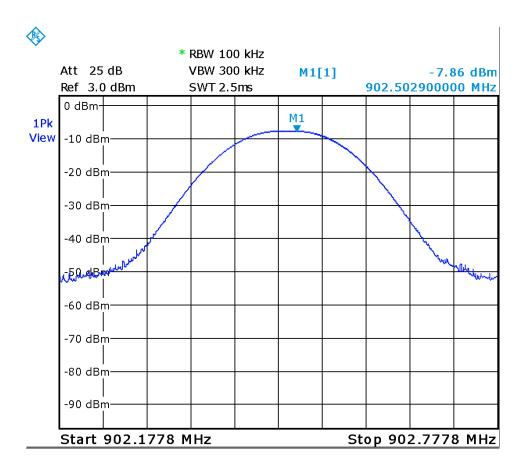
Low Channel Note: 20 dB for external attenuation losses added to value shown above.
