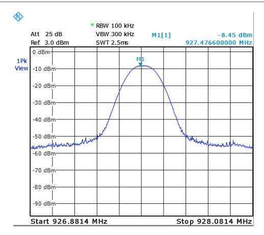
High Channel Note: 20 dB for external attenuation losses added to value shown above.
