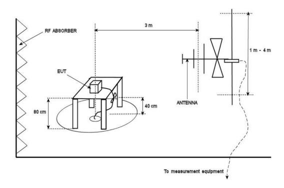
Note: In accordance with FCC Part 15, section 15.31(f)(1) testing was performed at a 3 meter test distance and an extrapolation factor of 10.5 dB was applied.
