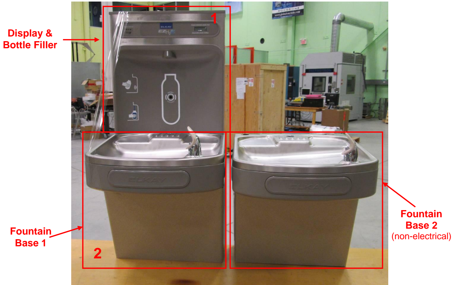
Photo 1. EUT – Bi-Level Water Fountain, External view. Single Level consists of 1 and 2 only.
