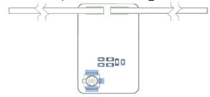
$\begin{array}{lll} \mbox{Frequency range:} & 2 \mbox{ 400 MHz} \\ \mbox{Impendance:} & 50 \Omega \\ \mbox{VSWR:} & <2:1 \\ \mbox{Peak Gain:} & 4.3 \mbox{ dBi} \end{array}$
