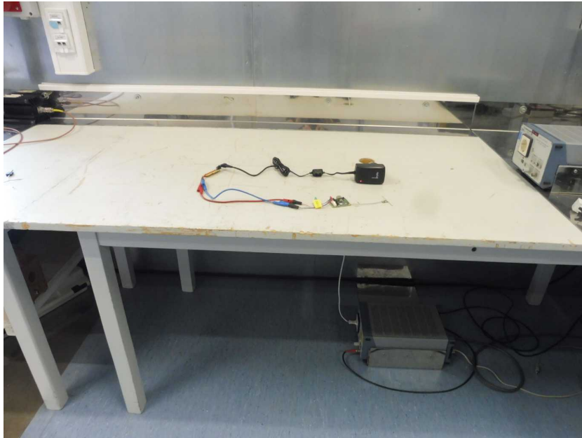
Photo 19: AC conducted emission test setup, 902-928 Proprietary
