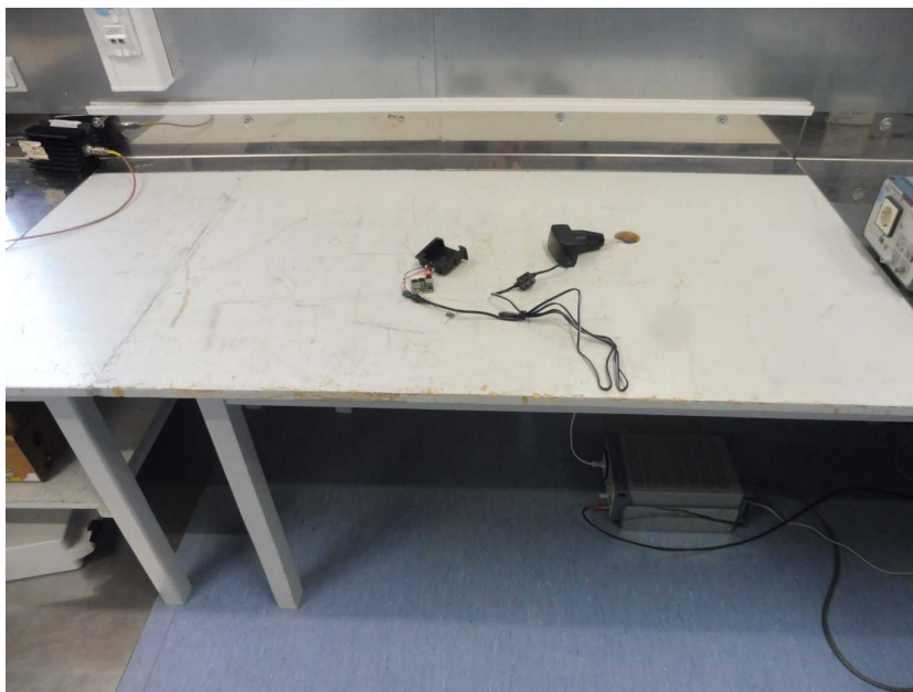
Photo 18: AC conducted emission test setup, BTLE
