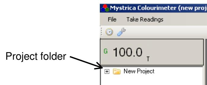
The left side of the screen displays, below the current readings and settings from the colorimeter, a list of the experiments and data sequences contained in the project folder, (double click the project folder and experiment files to view these).
