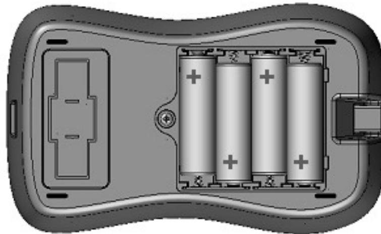
The unit uses 6V from four AA batteries. These are inserted by removing the screw on the battery holder.
