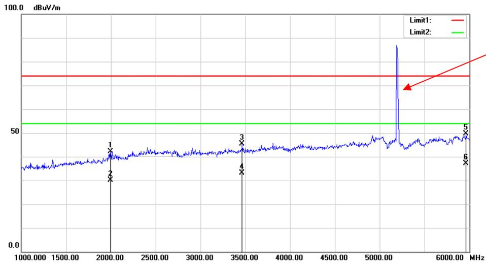
Fundamental Test with Band Rejection Filter
