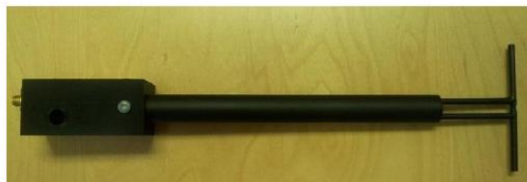
Figure 1 – MVG COMOSAR Validation Dipole
