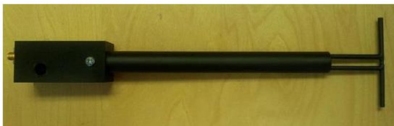
Figure 1 – MVG COMOSAR Validation Dipole
