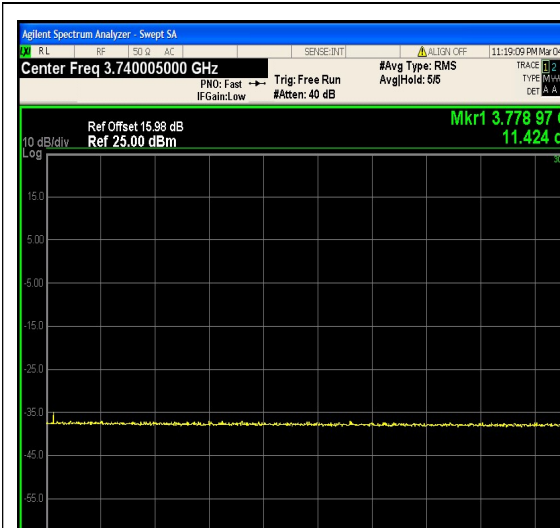
1-DC_2A_n77A-3700-3980-PC3-30-5+80-M+L-5-N/A-N/A-N/A-DFT-QPSK-Edge_1RB_Right-1@216-3700.005~3780.005(3778.965MHz, 11.424MHz, Limit30, Margin[18.576])-PASS-see graph
