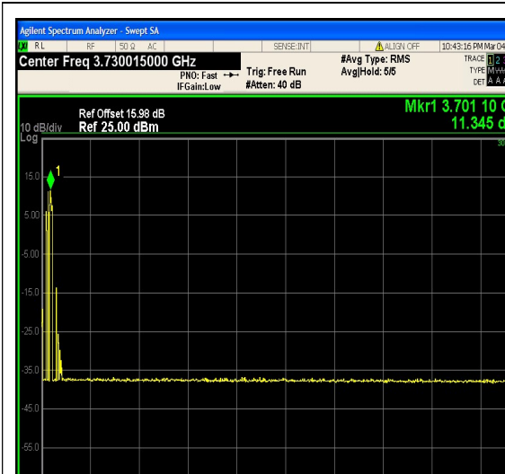
1-DC_2A_n77A-3700-3980-PC3-30-5+60-M+ L-1-N/A-N/A-N/A-DFT-PI2BPSK-Edge_1RB_ Left-1@0-3700.015~3760.015(3701.095MHz, 11.345MHz,Limit30,Margin[18.655])-PASS-se e graph
