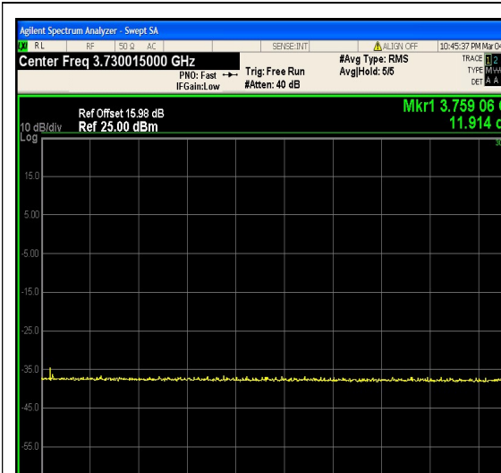
1-DC_2A_n77A-3700-3980-PC3-30-5+60-M+L-5-N/A-N/A-N/A-DFT-QPSK-Edge_1RB_Right-1@161-3700.015~3760.015(3759.055MHz, 11.914MHz, Limit30, Margin[18.086])-PASS-see graph
