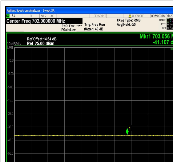
1-N12-PC3-15-10-L-1-DFT-PI2BPSK-Edge_1 RB_Left-1@0-Ant1-699.0~705.0(703.056MHz, -41.11MHz,Limit30,Margin[71.11])-PASS-see graph
