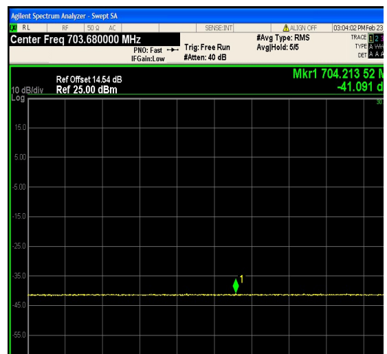
1-N12-PC3-15-10-L-6-CP-QPSK-Outer_Full- 52@0-Ant1-699.0~708.36(704.21352MHz,-4 1.09MHz,Limit30,Margin[71.09])-PASS-see graph
