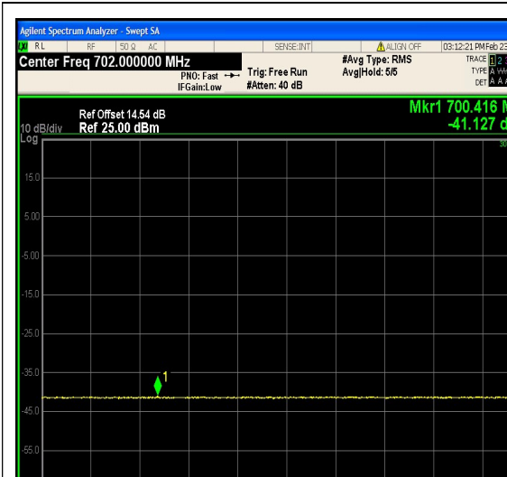
1-N12-PC3-15-15-L-1-DFT-PI2BPSK-Edge_1 RB_Left-1@0-Ant1-699.0~705.0(700.416MHz, -41.13MHz,Limit30,Margin[71.13])-PASS-se e graph
