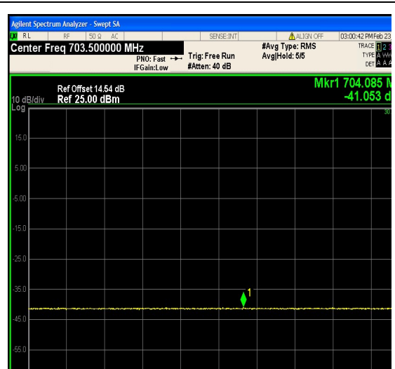
1-N12-PC3-15-10-L-3-DFT-PI2BPSK-Outer_ Full-50@0-Ant1-699.0~708.0(704.085MHz,-4 1.05MHz,Limit30,Margin[71.05])-PASS-see graph
