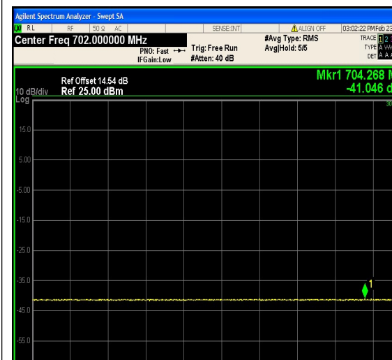
1-N12-PC3-15-10-L-4-CP-QPSK-Edge_1RB Left-1@0-Ant1-699.0~705.0(704.268MHz,-4 1.05MHz,Limit30,Margin[71.05])-PASS-see graph
