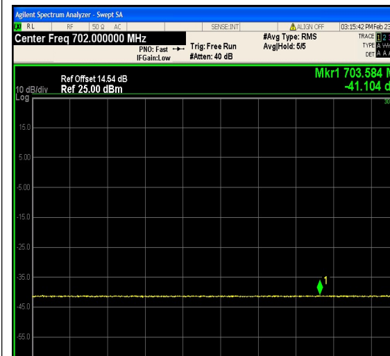
1-N12-PC3-15-15-L-4-CP-QPSK-Edge_1RB Left-1@0-Ant1-699.0~705.0(703.584MHz,-4 1.1MHz,Limit30,Margin[71.1])-PASS-see graph
