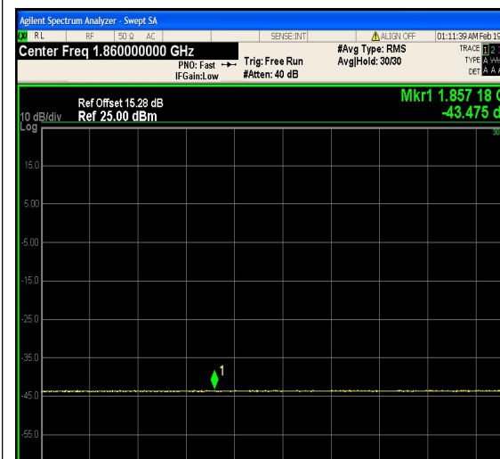
1-N25-PC3-15-20-L-4-CP-QPSK-Edge_1RB Left-1@0-Ant1-1850.0~1870.0(1857.18MHz ,-43.48MHz,Limit30,Margin[73.48])-PASS-se e graph
