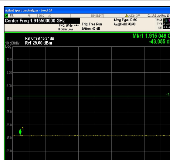
1-N25-PC3-15-20-H-3-DFT-PI2BPSK-Outer_Full-100@0-Ant1-1915.0~1916.0(1915.046MHz,-43.06MHz,Limit-13,Margin[30.06])-PASS-see graph
