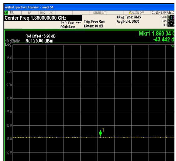
1-N25-PC3-15-20-L-6-CP-QPSK-Outer_Full- 106@0-Ant1-1850.0~1870.0(1860.34MHz,-4 3.44MHz,Limit30,Margin[73.44])-PASS-see graph
