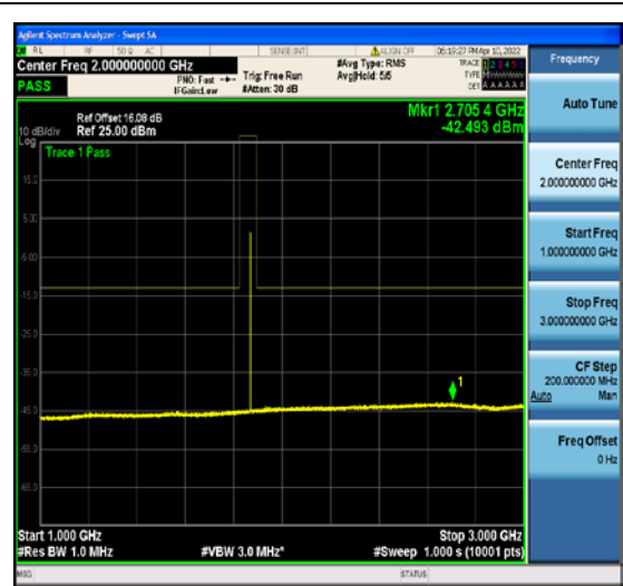
1-N2-PC3-15-20-L-5-DFT-QPSK-Edge_1RB_ Right-1 @ 105-1000-3000-Ant1--42.49--13-PA SS
