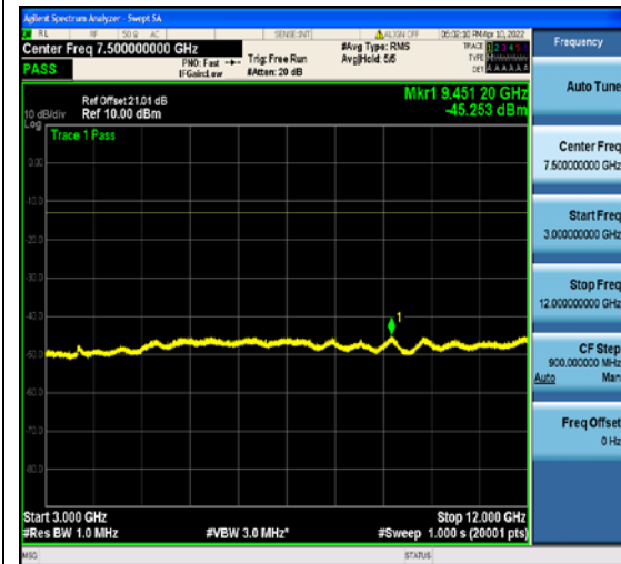
1-N2-PC3-15-10-H-5-DFT-QPSK-Edge_1RB _Right-1 @51-3000-12000-Ant1--45.25--13-P ASS
