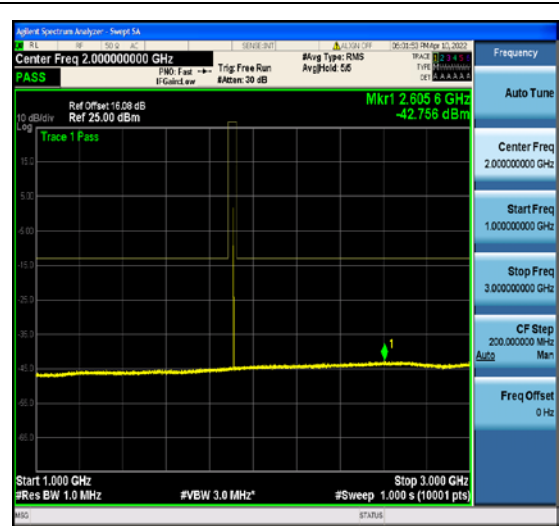
1-N2-PC3-15-10-H-5-DFT-QPSK-Edge_1RB _Right-1 @51-1000-3000-Ant1--42.76--13-PA SS
