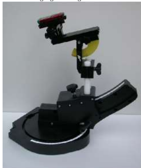
Device holder supplied by SPEAG
