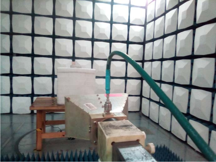
Radiated Emission Above 1GHz View
