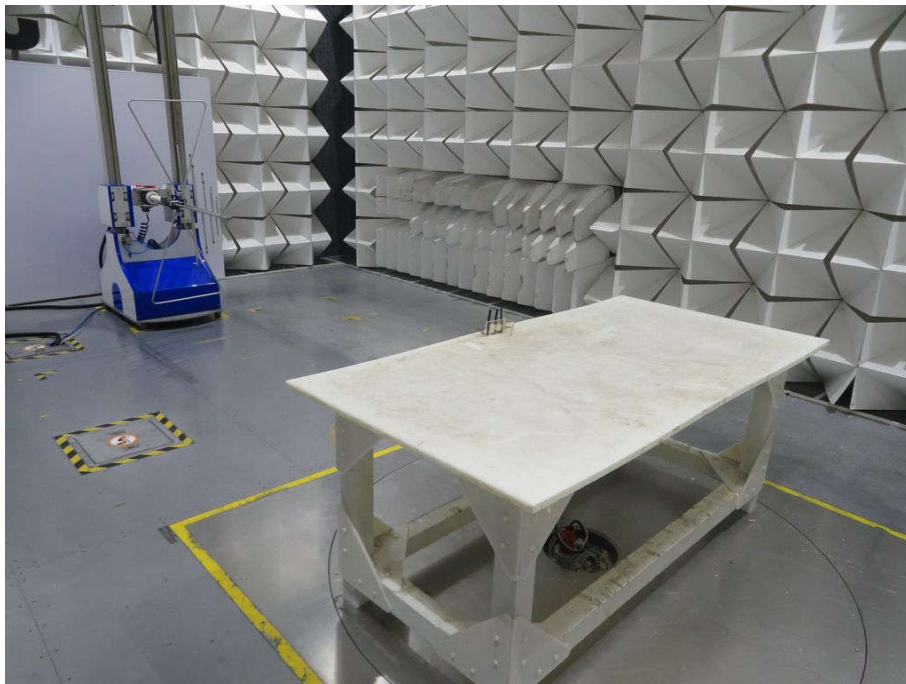
Radiated spurious emission Test Setup-2(Below 1GHz)
