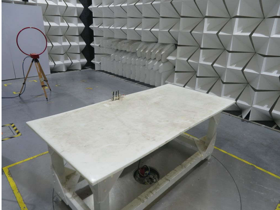
Radiated spurious emission Test Setup-1( Below 30MHz)
