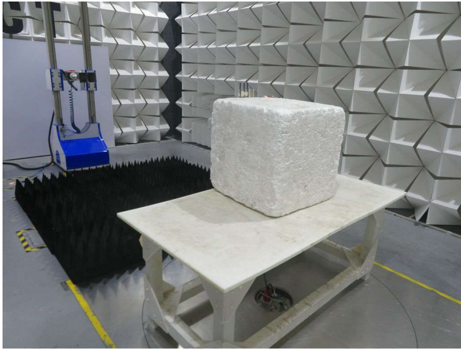
Radiated spurious emission Test Setup-3(Above 1GHz)
