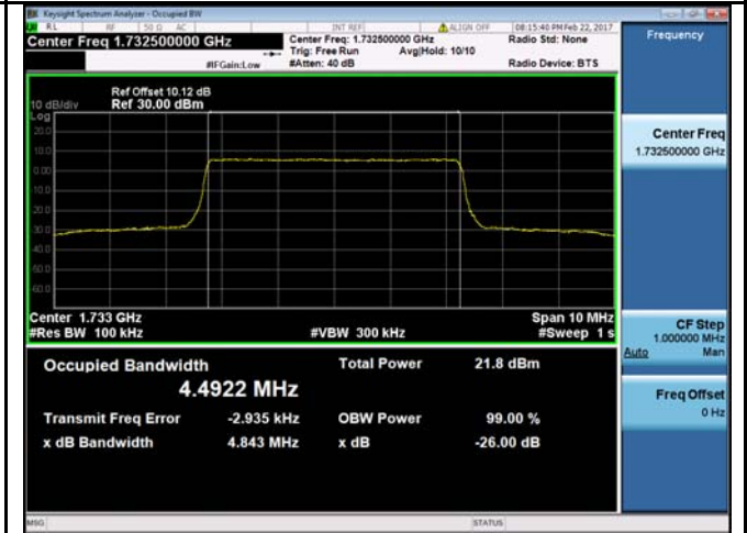
LTE band 4 - Middle CH 16QAM-5
