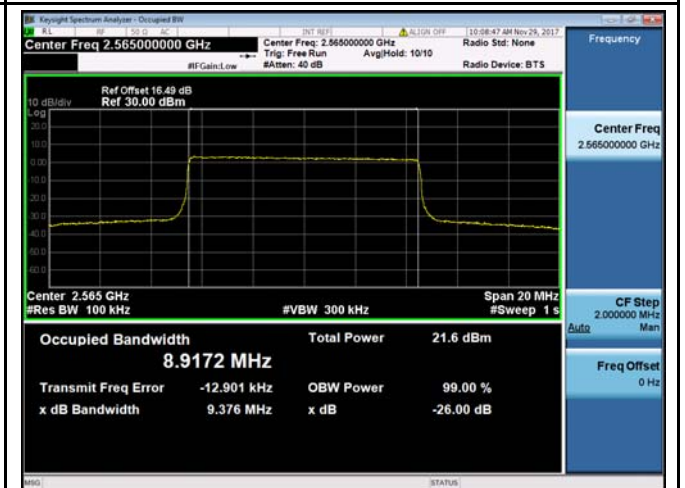
LTE band 7 - Middle CH 16QAM-10
