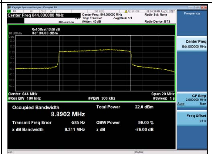
LTE band 5 - Middle CH 16QAM-10
