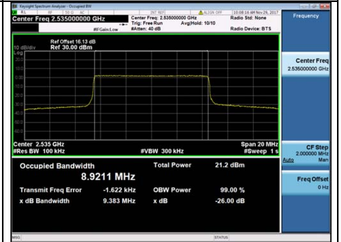
LTE band 7 - Middle CH 16QAM-10
