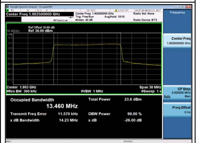
LTE band 2 - Middle CH 16QAM-15
