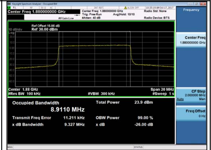
LTE band 2 - Middle CH 16QAM-10
