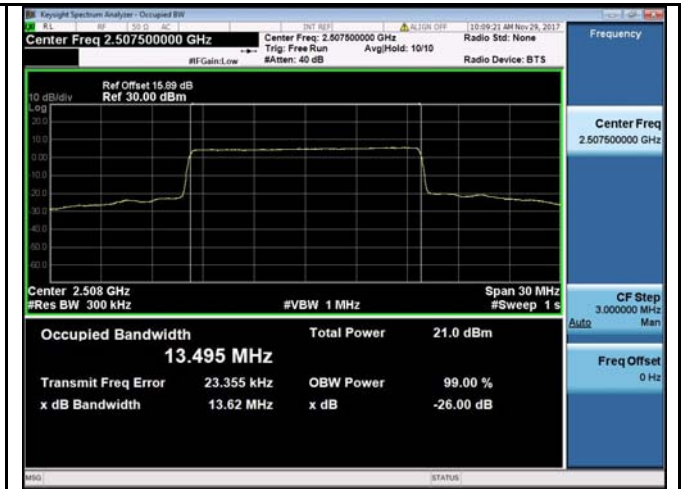
LTE band 7 - Low CH 16QAM-15
