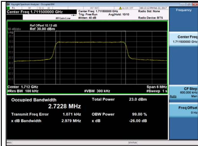
LTE band 4 - Low CH QPSK-3
