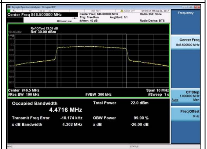
LTE band 5 - Middle CH 16QAM-5
