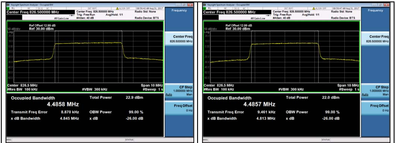
LTE band 5 - Low CH QPSK-5
