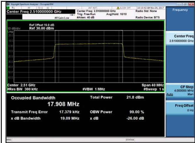
LTE band 7 - Low CH QPSK-20
