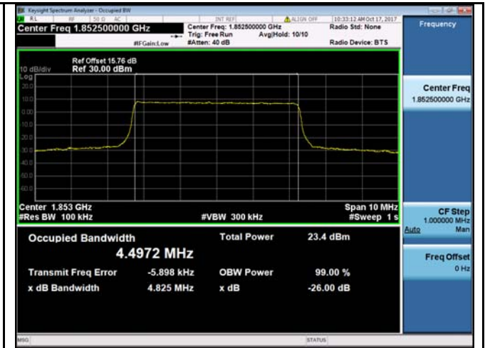
LTE band 2 - Low CH 16QAM-5
