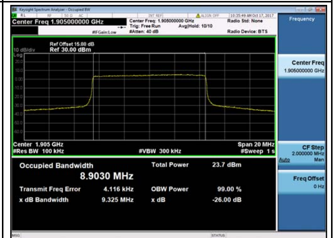
LTE band 2 - Middle CH 16QAM-10
