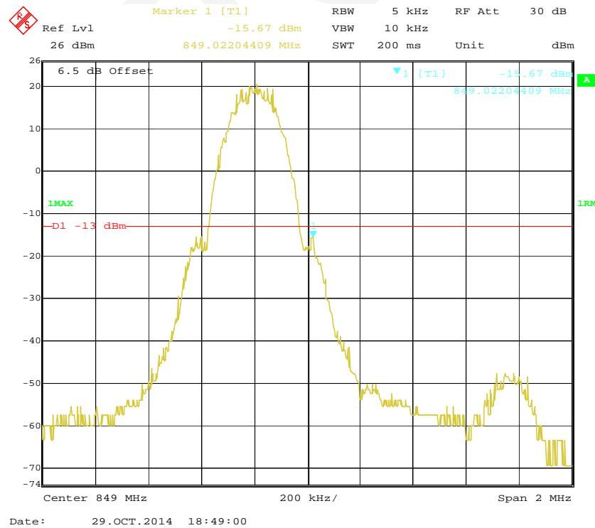
**Cellular Band, Left Band Edge for EGPRS Mode**
