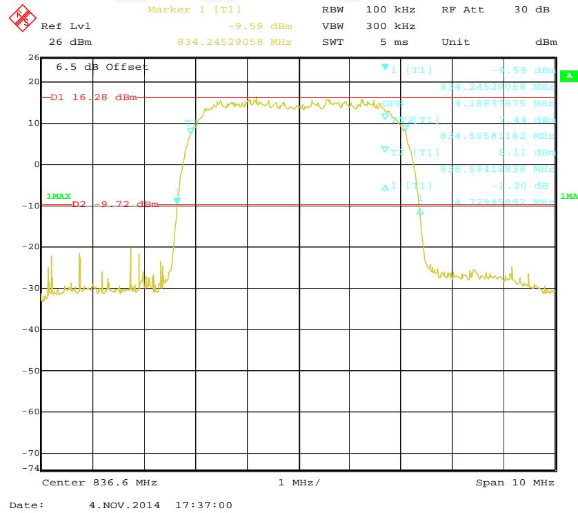
**99% Occupied & 26 dB Emissions Bandwidth for HSUPA (BPSK) Mode (Antenna 1)**
