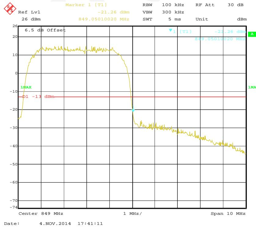
**PCS Band, Left Band Edge for GSM (GMSK) Mode**
