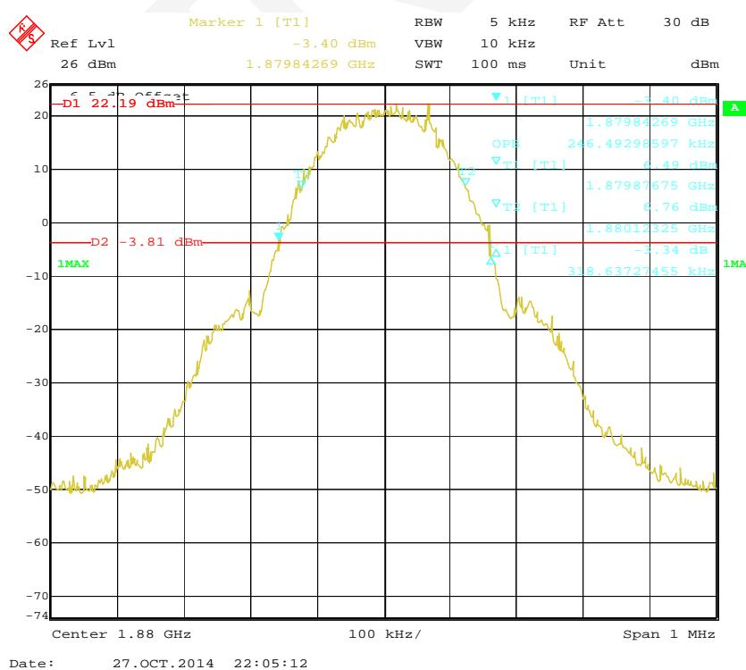
**99% Occupied & 26 dB Emissions Bandwidth for EGPRS Mode (Antenna 1)**
