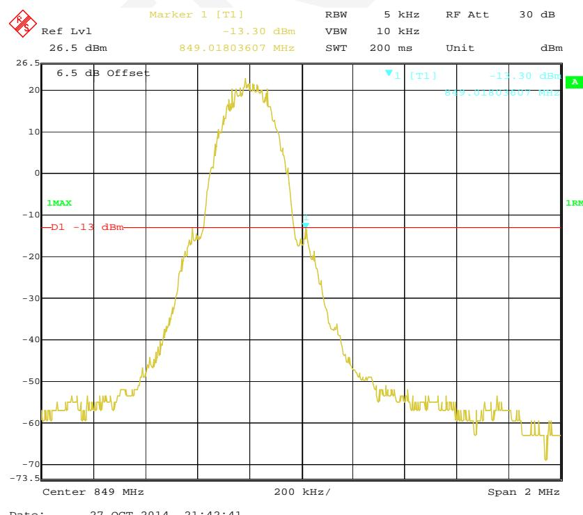
**Cellular Band, Left Band Edge for EGPRS Mode**
