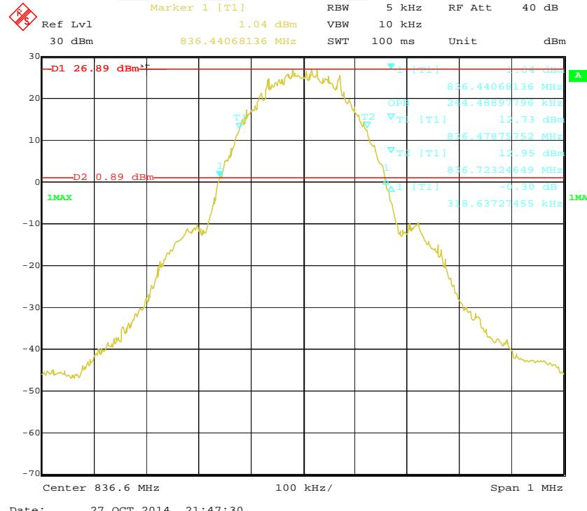
**99% Occupied & 26 dB Emissions Bandwidth for EGPRS Mode (Antenna 1)**
