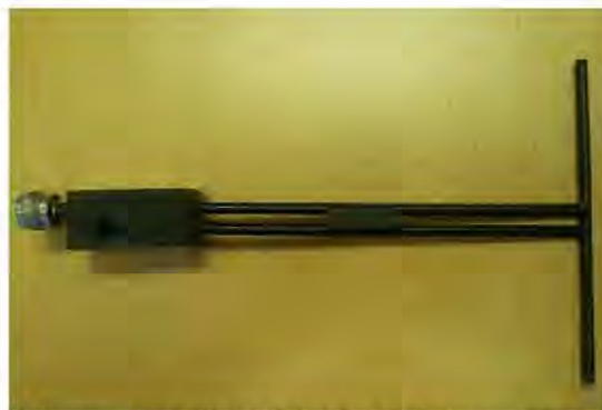
Figure 1 – MVG COMOSAR Validation Dipole
