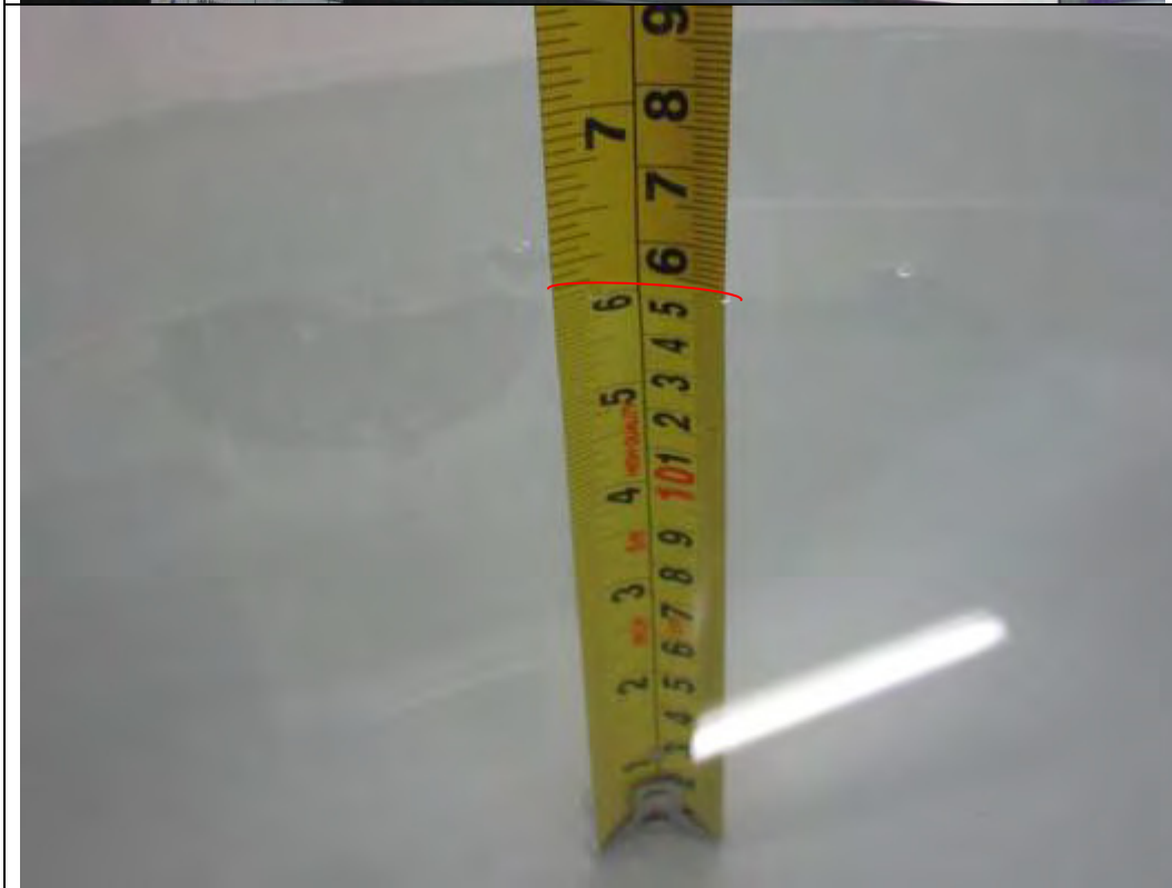
Liquid depth \geq 15cm
