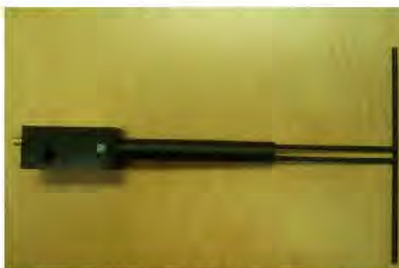
Figure 1 – MVG COMOSAR Validation Dipole
