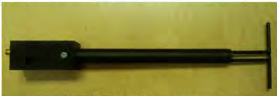
Figure 1 – MVG COMOSAR Validation Dipole
