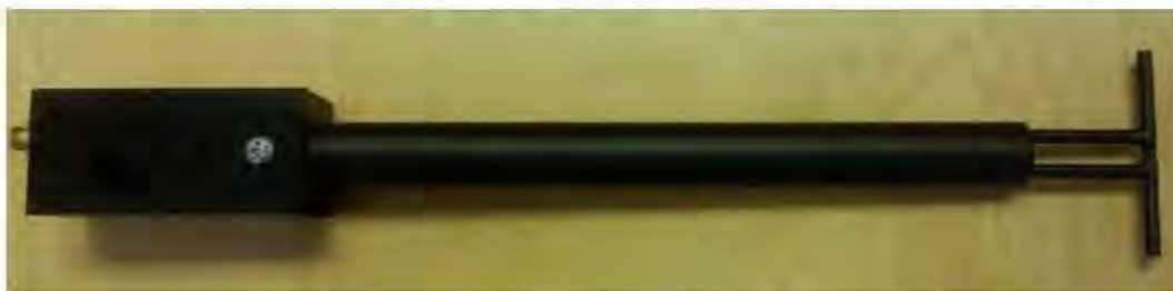
Figure 1 – MVG COMOSAR Validation Dipole
