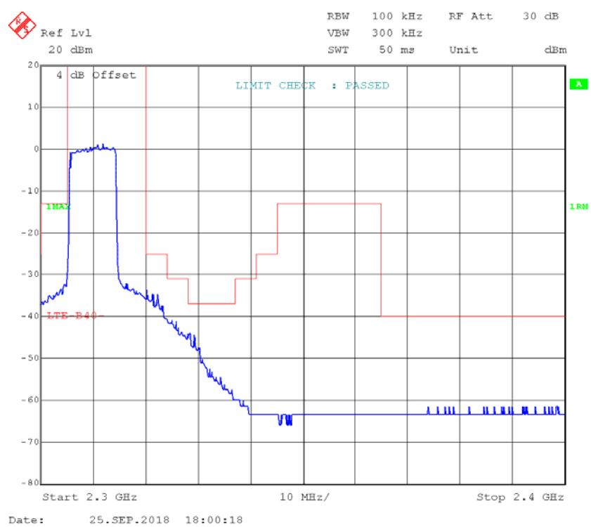
**LTE Band 40(2350-2360MHz)****QPSK\_5MHz\_25 RB\_Left**
