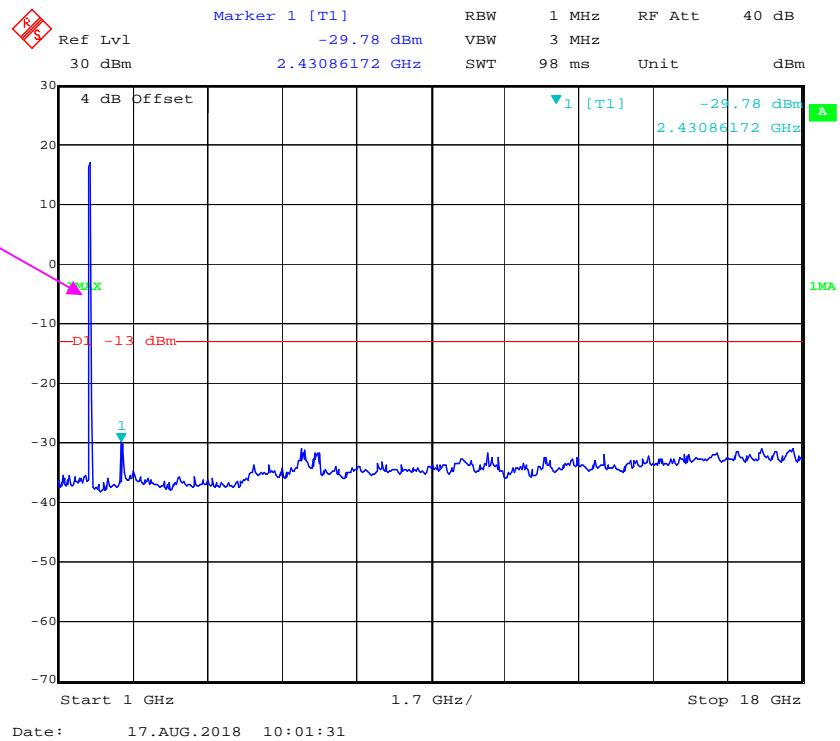
**LTE Band 5 (Middle Channel)****QPSK\_1.4 MHz**
