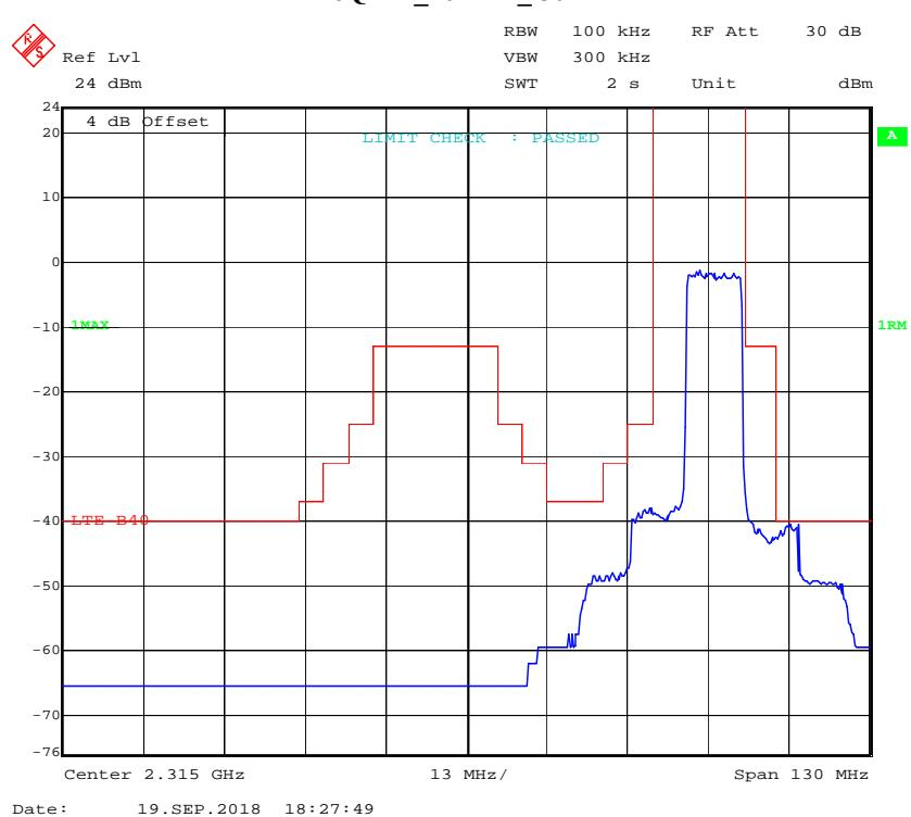
**LTE Band 41****QPSK\_5MHz\_25 RB\_Left**
