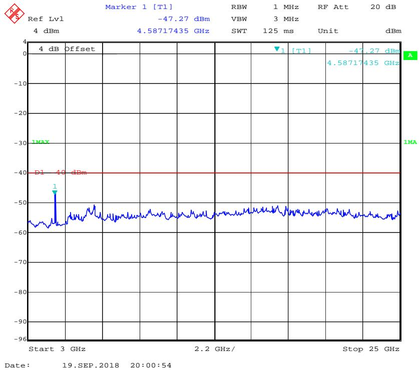
**LTE Band 40 (2350-2360MHz Middle Channel)****QPSK\_5 MHz**
