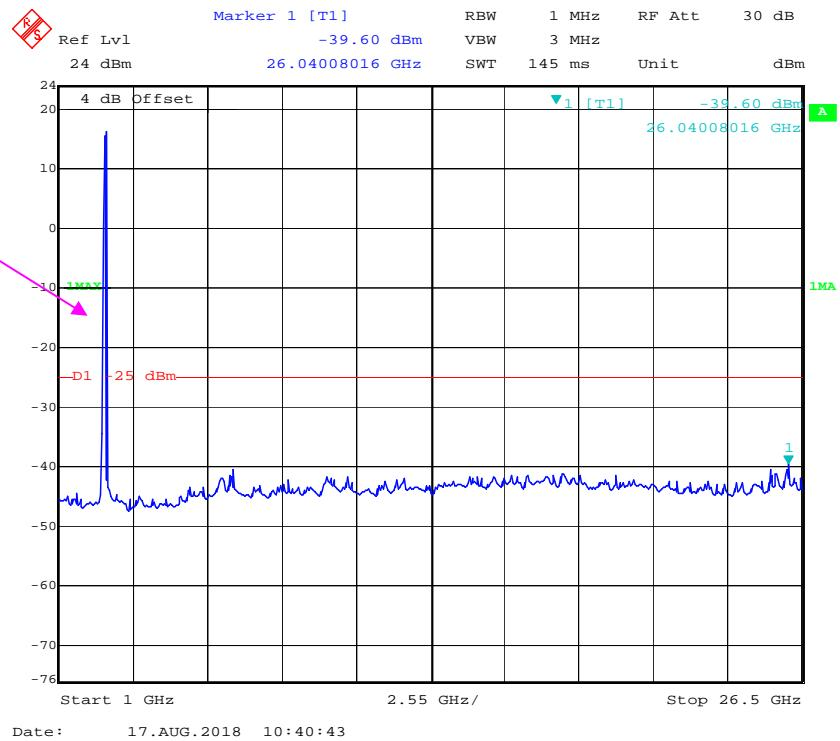
**LTE Band 40 (2305-2315MHz Middle Channel)****QPSK\_5 MHz**
