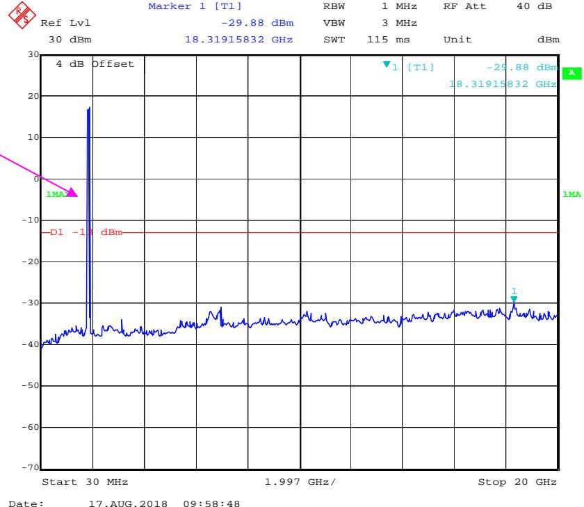
**LTE Band 4 (Middle Channel)****QPSK\_1.4 MHz**
