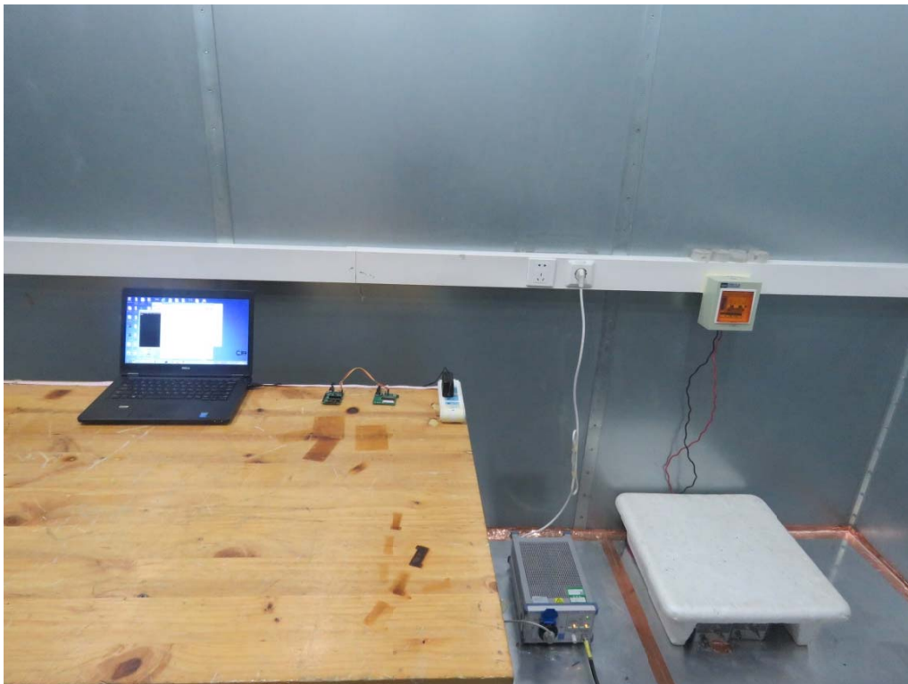
Picture 2 Conducted Emission Test Setup
