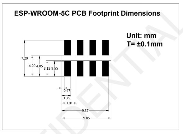
Figure 8-1. Recommended PCB Land Pattern of ESP-WROOM-5C
