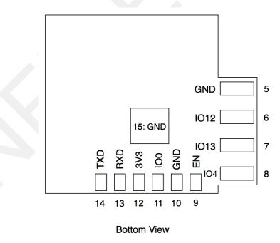
Figure 2-2. ESP-WROOM-5C Pin Layout (Bottom View)
