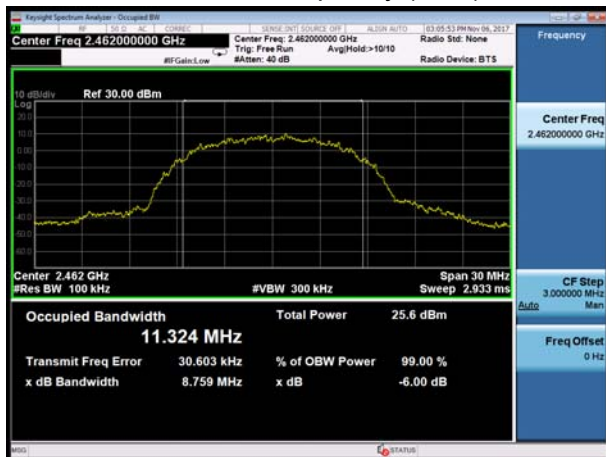
802.11b, Carrier frequency (MHz): 2462
