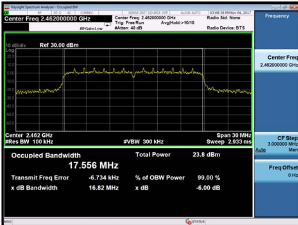
802.11n(HT20), Carrier frequency (MHz): 2462
