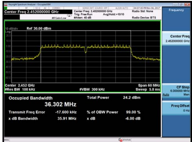
802.11n(HT40), Carrier frequency (MHz): 2452
