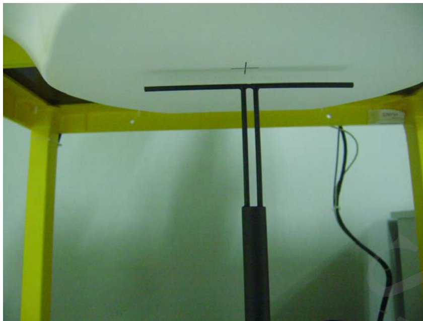
Setup Photo of Dipole Antenna
