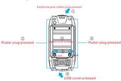
\* In order to be waterproof and dustproof, please ensure battery cover, battery lock catch, screw cover, earphone jack cover and USB rubber cover are in perfectly close status. This will not be specially declared in below content.
