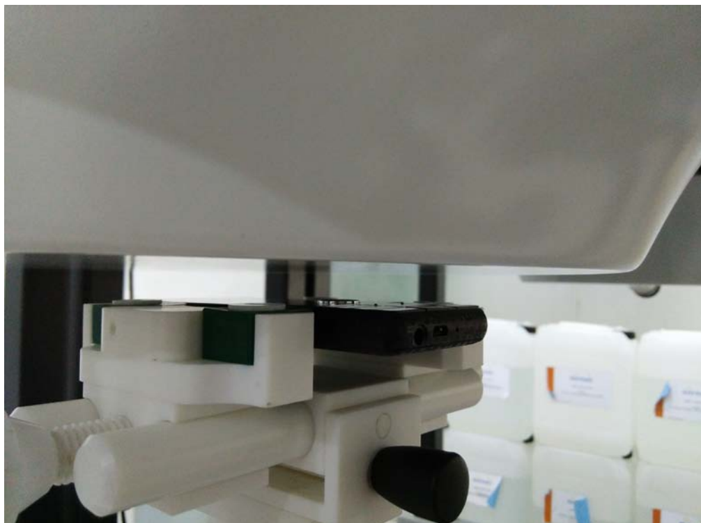
Body Front side(separation distance is 10mm)
