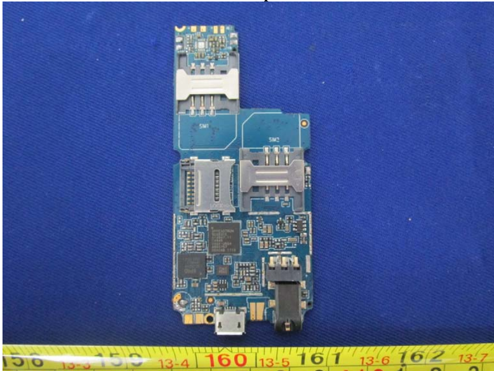
EUT –Mainboard Top Unshield View
