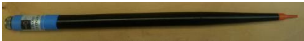
Figure 1 – MVG COMOSAR Dosimetric E field Dipole
