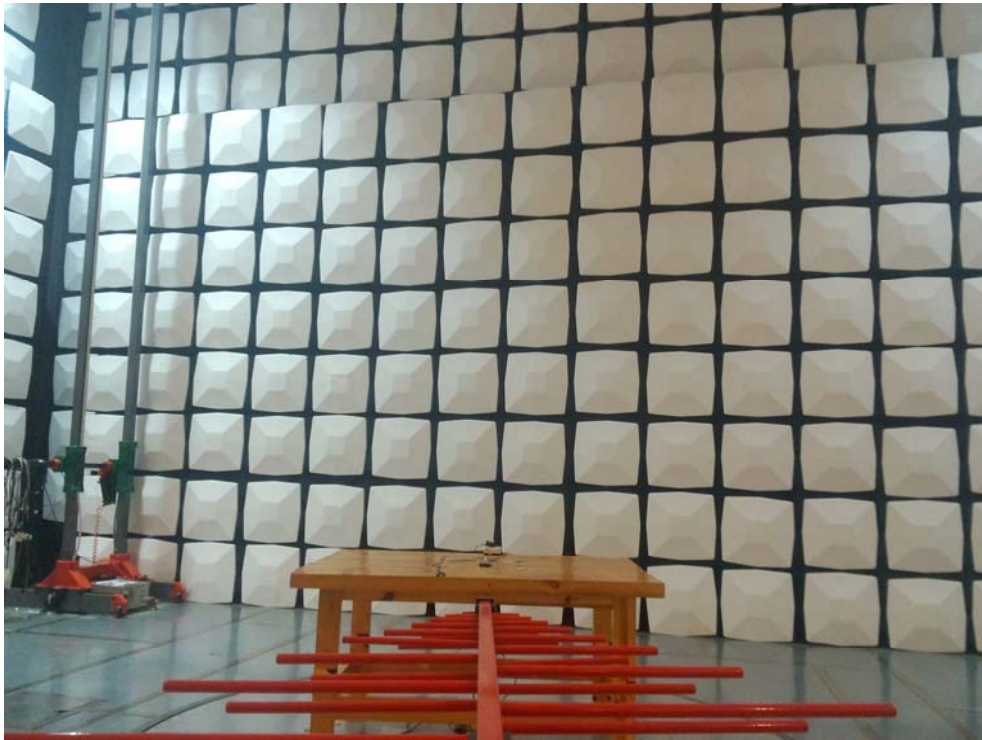
Radiated Emission View (Below 1GHz)
