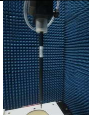
Fig. 8.2 Photo of E-Field Probe
