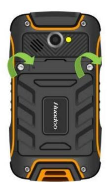
Turn the screw lock to the right on the battery cover till it locks.
